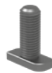
Art. 0129 Hammerhead screws 28/15 Measurements: M8 16 ±70 M10 16 ±100 Use: Mounting Rail Art. 0110 Material: A2 1.4301 stainless steel
