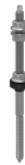
Art. 0121 Hanger Bolt With nuts and EPDM sealing washer M10 160 ±300 M12 200 ±400 Use with Art. 0122 or Art. 045 Use: metal roof/eternit roof Material: A2 1.4301 stainless steel
